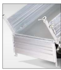
**Tough. Tougher. Steel:** The robust, hotdip galvanised steel sidewalls (400 mm high) are designed for the toughest applications.
